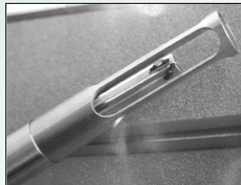
Probe Microflown 3D type USP
